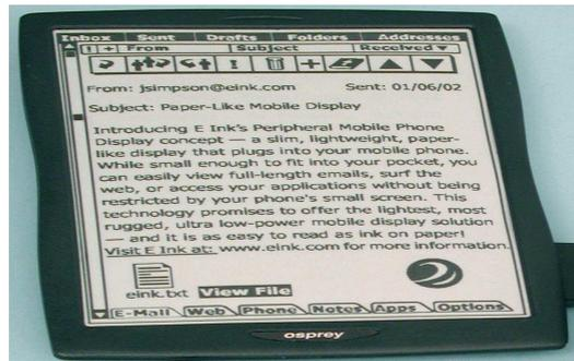
**Figure 5.4: An Electronic Display Screen for a PDA Device Using E-Ink**
