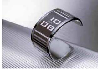
**Figure 5.1: World's First Watch to Utilize an Electronic Paper Display**
